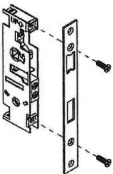
**STEP 1 - REMOVE MORTISE PLATE.** IF SPACERS ARE BEING USED, INSTALL THE LIVEBOLT SPACER ONTO THE THREADED SIDE OF THE LIVE BOLT.
