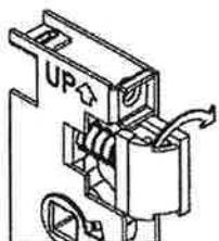
**STEP 2 - INSERT LIVE BOLT NUT THROUGH THE BACK OF THE BODY.** PUT THE LIVE BOLT SPRING ON THE THREADED PART OF THE LIVE BOLT, AND SCREW IT INTO THE LIVE BOLT NUT. CONTINUE TO SCREW LIVE BOLT TOGETHER UNTIL IT CANNOT BE TIGHTENED FURTHER. IF USING THE SPACER, THE SPACER SHOULD BE TOUCHING THE LIVE BOLT NUT, IF NOT USING THE SPACER, NO THREADS SHOULD BE VISIBLE.
