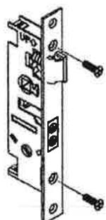
**STEP 3 - ENSURE THAT THE LIVE BOLT IS FACING THE CORRECT DIRECTION.** IF IT IS NOT FACING THE CORRECT DIRECTION, UNSCREW IT ONE HALF TURN SO THAT IT IS FACING THE CORRECT DIRECTION. ATTACH THE MORTISE PLATE AND INSTALL.
